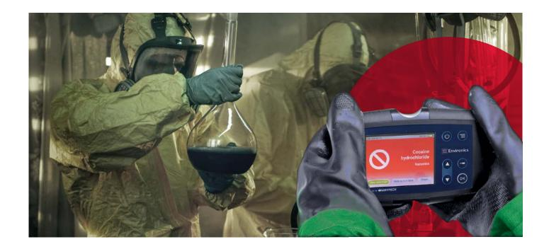
The 100 ID perfectly represents how a complex technology can be made easy to use. As a handheld Raman spectrometer, 100 ID is made for identifying a broad range of chemical compounds such as: explosives, narcotics, hazardous substances, chemical warfare agents (CWA) and pharmaceuticals.
