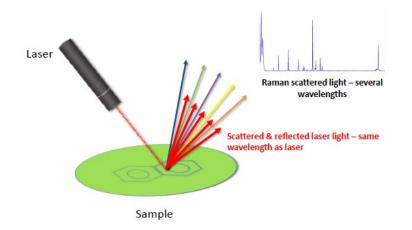
Raman spectroscopy is suitable for measuring inorganic and organic compounds in liquid or solid form. It does not detect gases or vapors. The sample can be analyzed directly through the wall of the sample container provided the container is clear.
