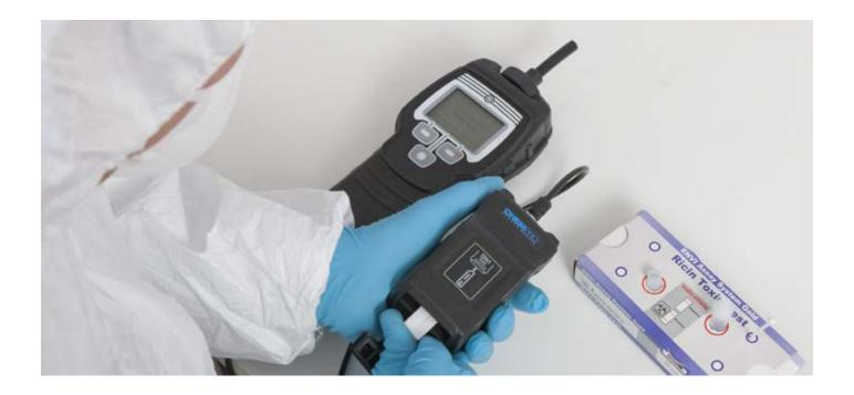
ENVI Assay System biodefence tests provide military and civil defence officers with a fast, simple and reliable solution for provisional, BWA identification from environmental samples.
