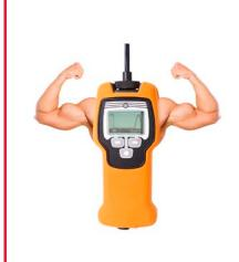
**The ChemPro100i** is a" PID on Steroids". With its 60,000-eV ionization energy it allows detection of hundreds of dangerous chemicals and then sorts the ions, instead of counting them like a PID. Therefore, the ChemPro100i 100i is ideally suitable to warn the presence of dangerous gases. The detection technology is based on orthogonal sensors with a 16 channel IMS and multiple other sensors.
