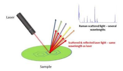
Raman spectroscopy is suitable for measuring inorganic and organic compounds in liquid or solid form. It does not detect gases or vapors. The sample can be analyzed directly through the wall of the sample container provided the container is clear.
